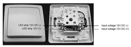
Upon request, a dimmer can be built-in into any switch, so you can choose any design to match the other switches and sockets in the room. We will either agree to the type of switch which is delivered by us, or you can send your switch into which we will build in the dimmer and will send it back or we will send you the dimmer module which you can build into the switch yourself.
