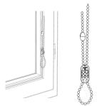
APPLY ONE HALF OF THE COUPLER TO EACH END OF THE CHAIN AND THEN LOCK BOTH COUPLER HALVES.
